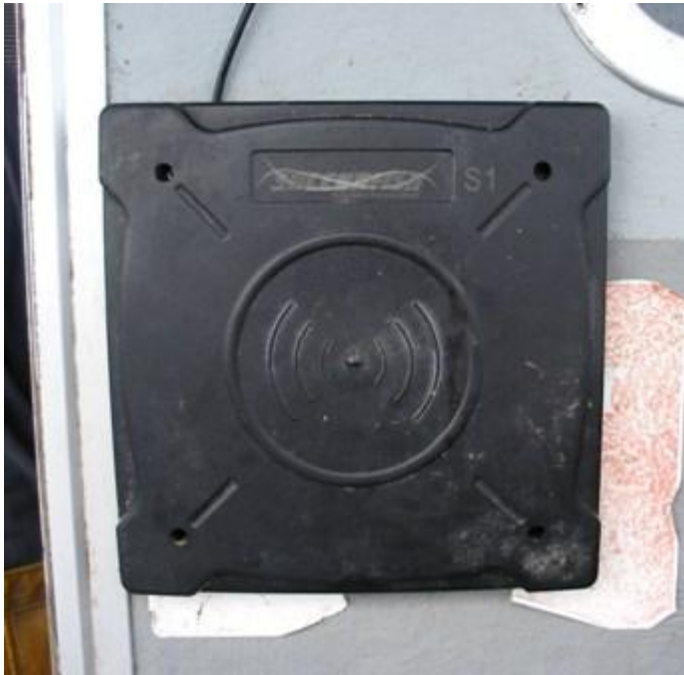
Figure 63. RFID reader fitted to a bulkhead close to pot hauler
